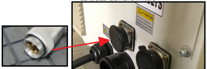
Fig 1.7 Matching connector that will plug into the controller box (shown left)
