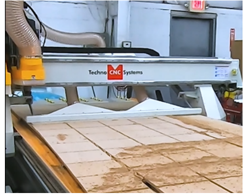
Pusher/Sweeper OFFLOADS MATERIAL
